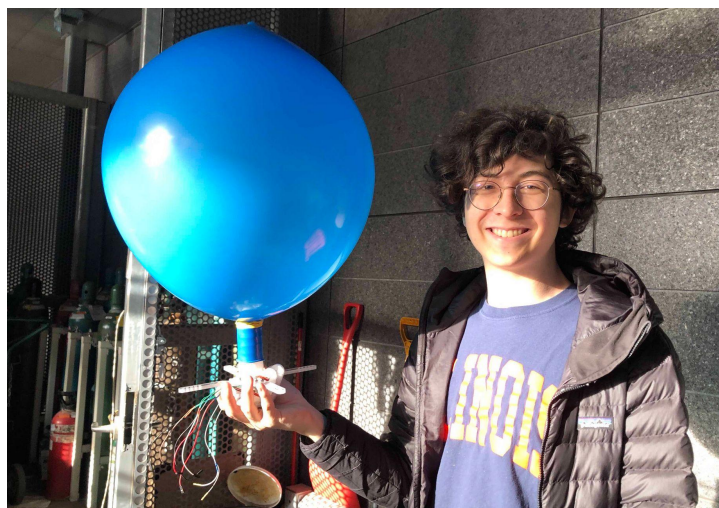
Figure 11: Testing the vent assembly with helium by the ECEB tank cage
