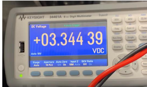
Figure 16. Verification of the Voltage drop to 3.3 V
