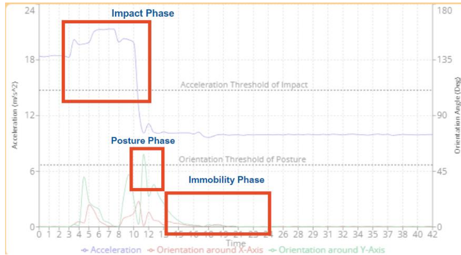
Figure 3. The three phases of the fall detection algorithm
