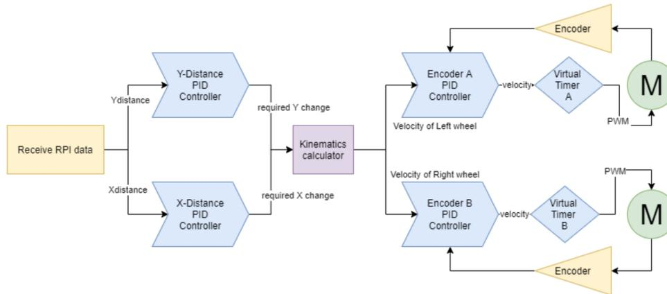
Figure 12) Finalized Block Diagram of Microcontroller Subsystem
