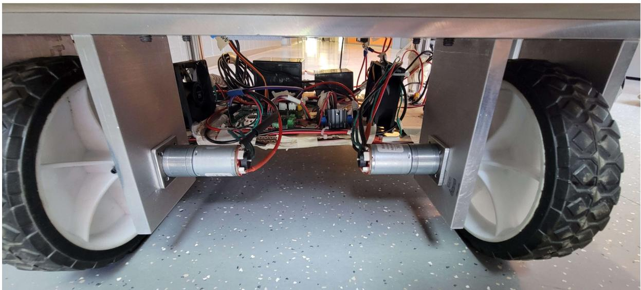
Figure 13) Back view of robot: motors, main circuit, cooling fans and batteries
