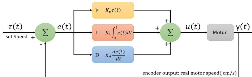
Figure 7) PID Speed Controllers
