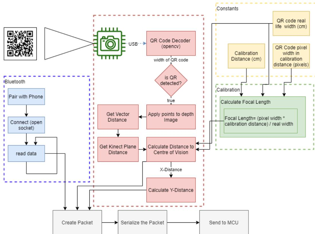
Figure 3) Detailed block diagram of RPI subsystem
