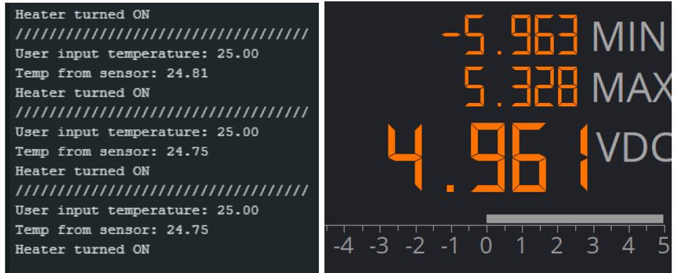
Figure 13: voltage drop between the heating element when GPIO 5 is HIGH
