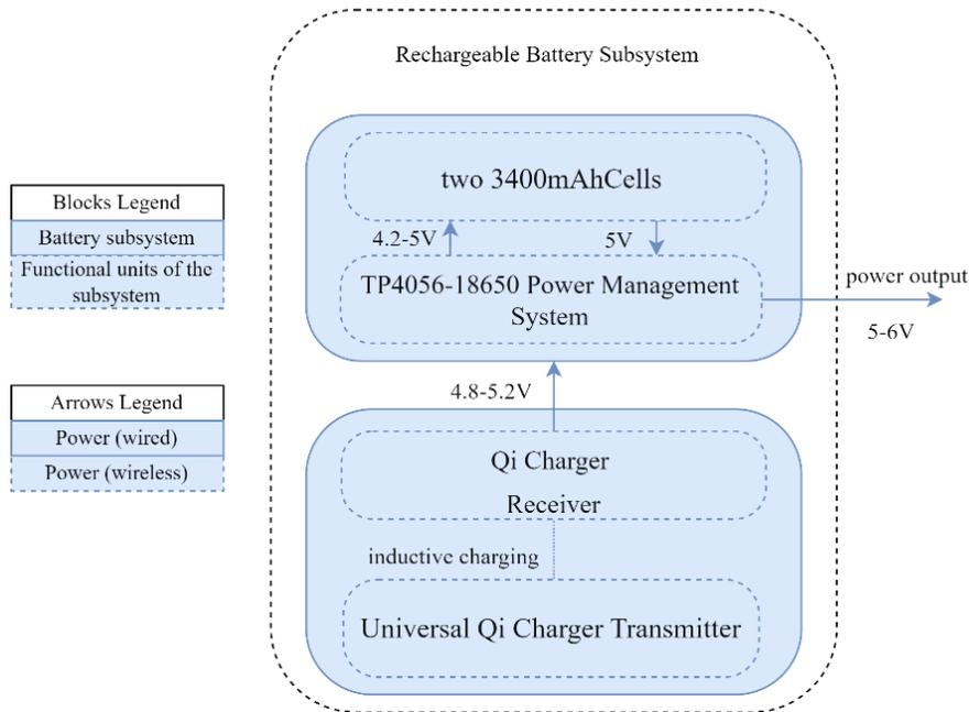
Figure 5: Modular block diagram of the rechargeable battery subsystem.
