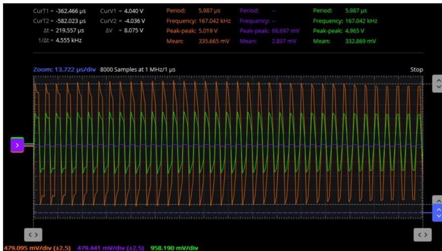
Figure 14: Voltage trace of the Qi transmitter terminals
