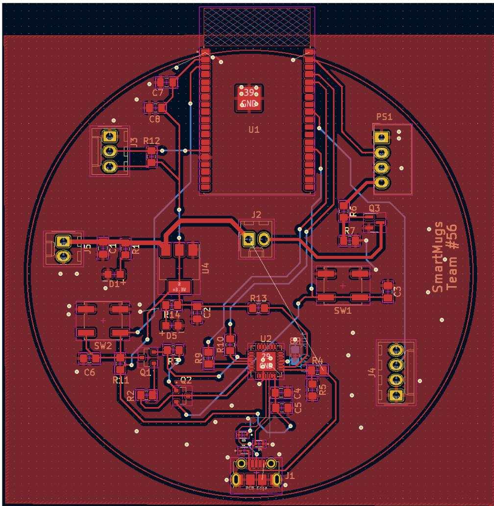
Figure 16: The smart mug PCB prototype.
