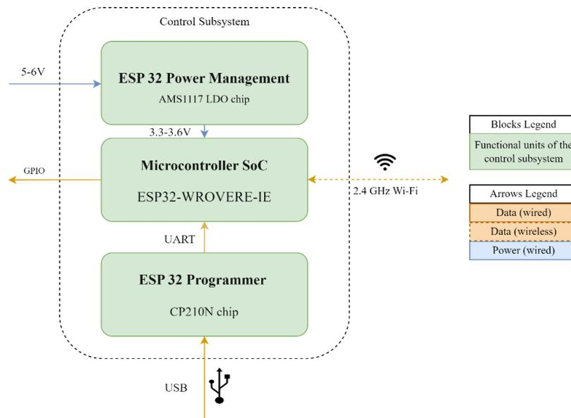
Figure 7: Modular block diagram of the control subsystem.
