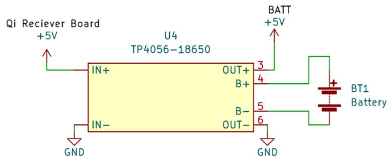
Figure 6: Circuit schematic diagram of the battery management system.
