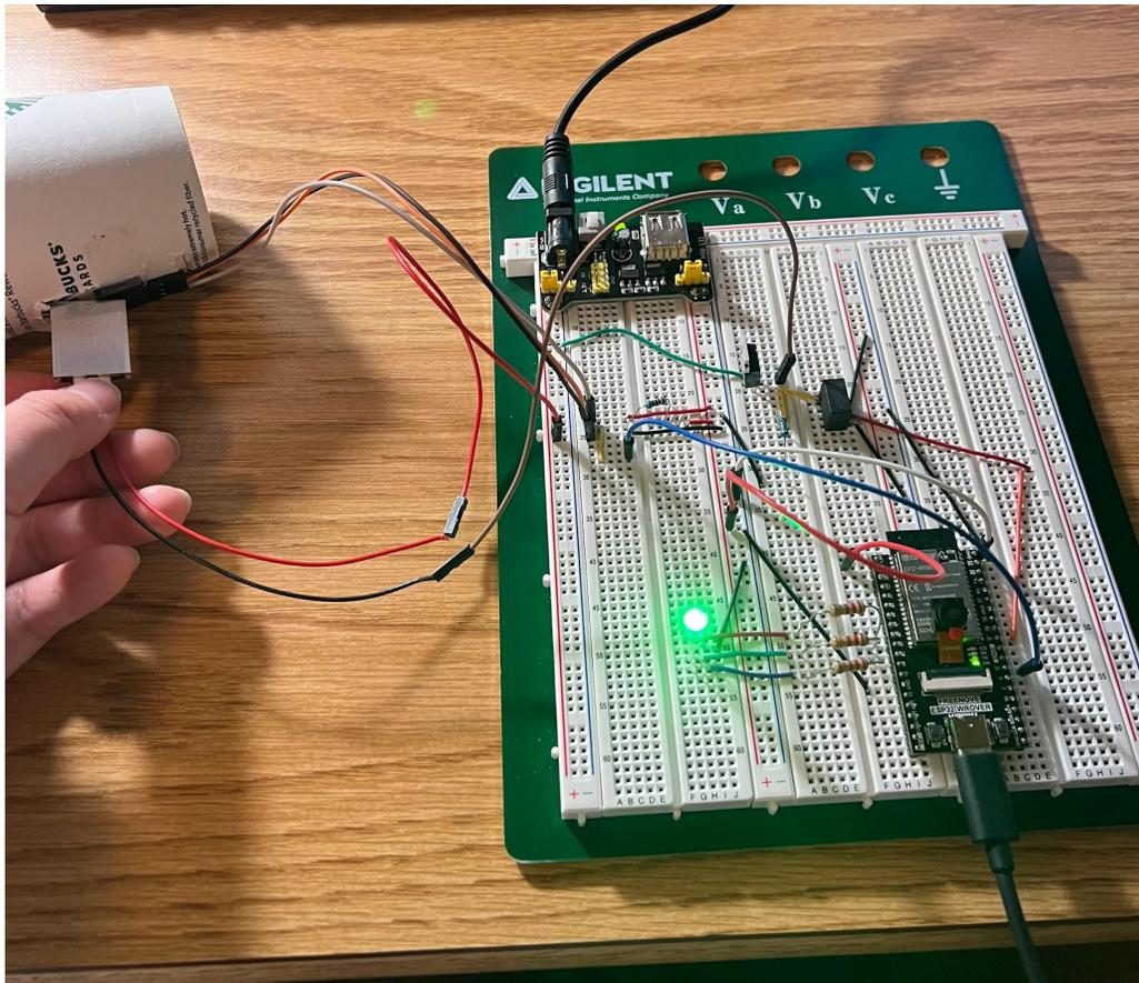
Figure 17: The breadboard circuit when the temperature reached the desired temperature.
