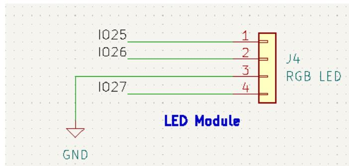
Figure 4: LED module schematics
