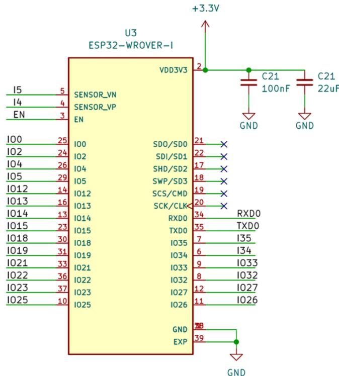
Figure 8: ESP32-WROVER-IE schematic diagram as connected in our device.
