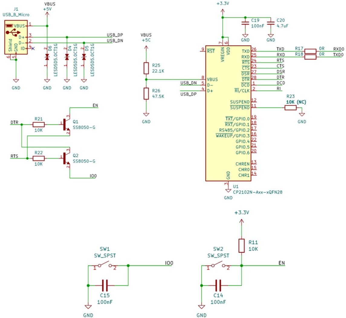
Figure 9: The ESP32 programmer circuit schematic diagram.
