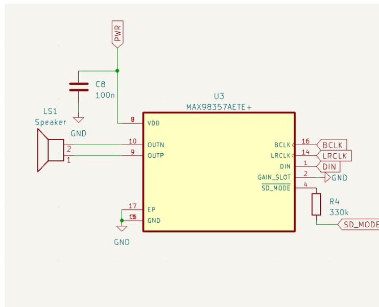
Fig. 4. Transducer Subsystem Schematic
