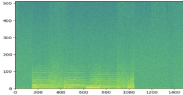
Fig. 6. STFT of sampled AUDIO signal sent to ESP32
