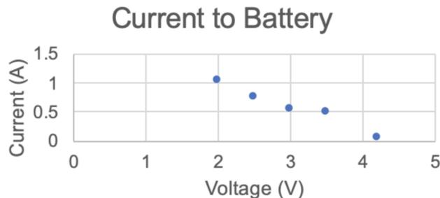
Fig. 5. Graph of Current vs Voltage delivered to the battery
