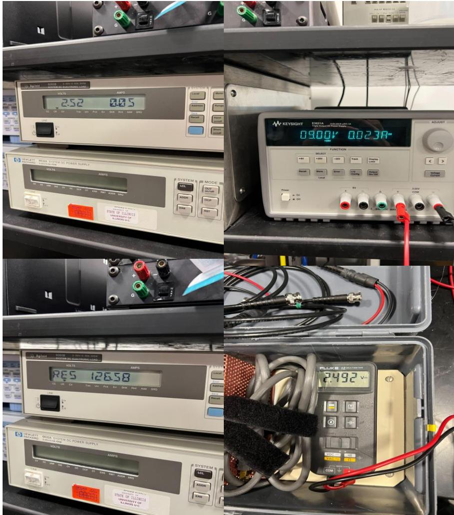
*Figure A5: 2.5V regulator readings. The top left is the electronic load readings. The top right is the power source readings. The bottom left is the electronic load resistance. The bottom right is the voltage read across the Vout and ground pins of the SPX1117.*
