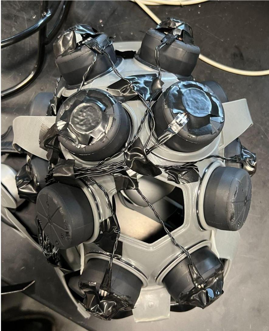
*Figure 9: FSR placement within helmet with spacers*
