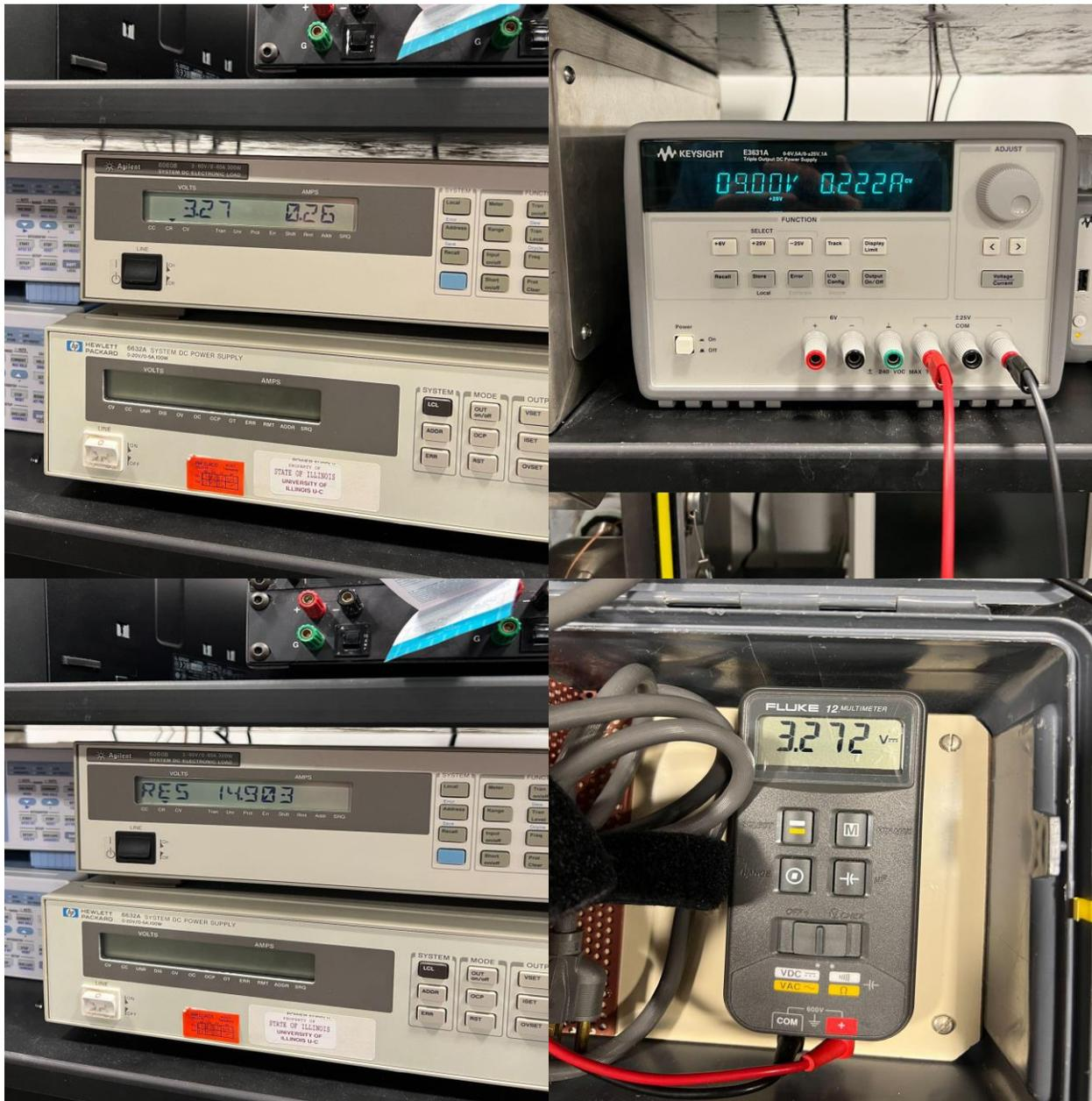
Figure A7: 3.3V regulator readings. The top left is the electronic load readings. The top right is the power source readings. The bottom left is the electronic load resistance. The bottom right is the voltage read across the Vout and ground pins of the SPX1117.
