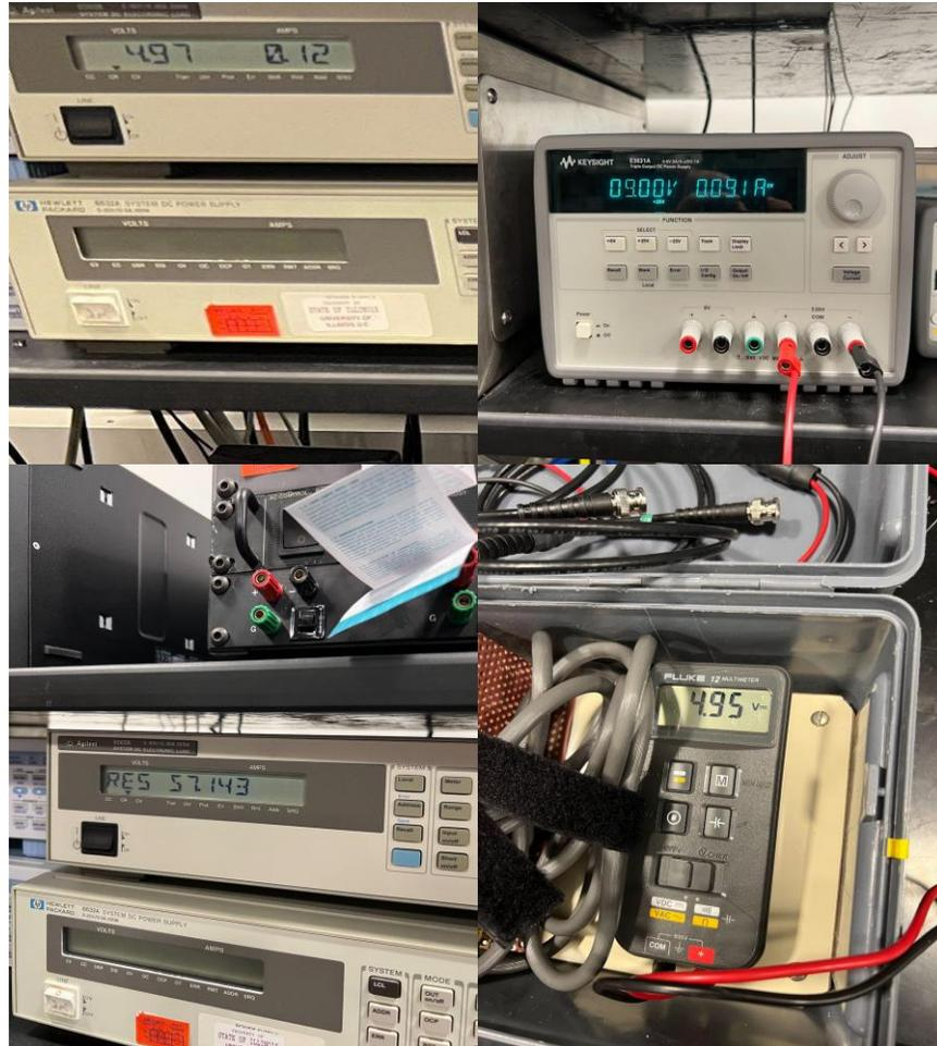
*Figure A8: 5V regulator readings. The top left is the electronic load values. The top right is the power source. The bottom left is the resistance the electronic load was set to. The bottom right is the reading across the Vout and ground pins of the SPX1117.*
