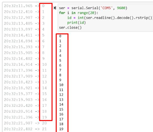
*Figure C1: The left image is the data being sent from the Arduino. The right image is the data as received by the COM port in the Python script.*
