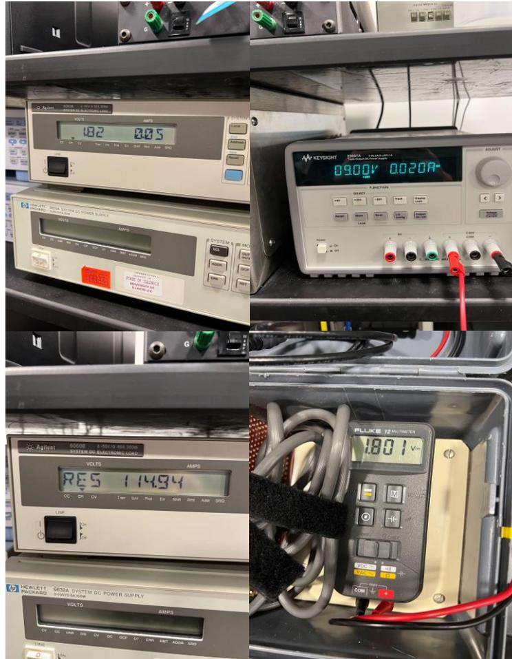
*Figure A4: 1.8V regulator testing readings. The top left is the electronic load readings. The top right is the power source readings. The bottom left is the electronic load resistance. The bottom right is the voltage read across the Vout and ground pins of the SPX1117.*
