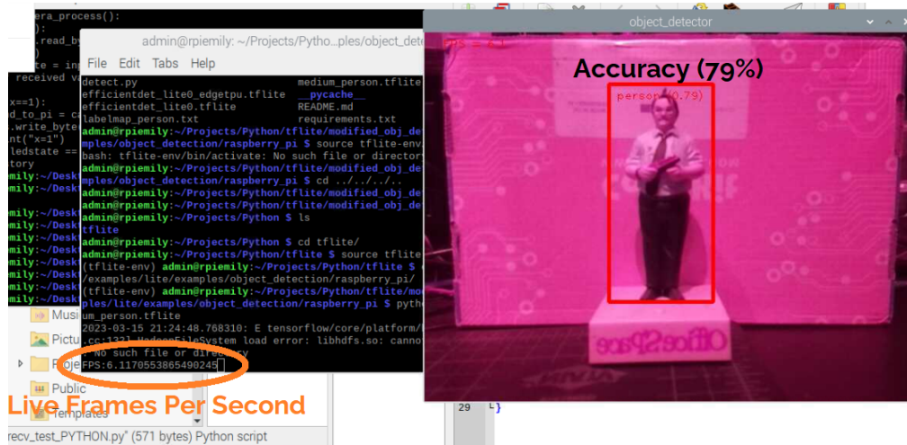
Figure 2.3.4: Object detection model using 500 training images on EfficientDet
