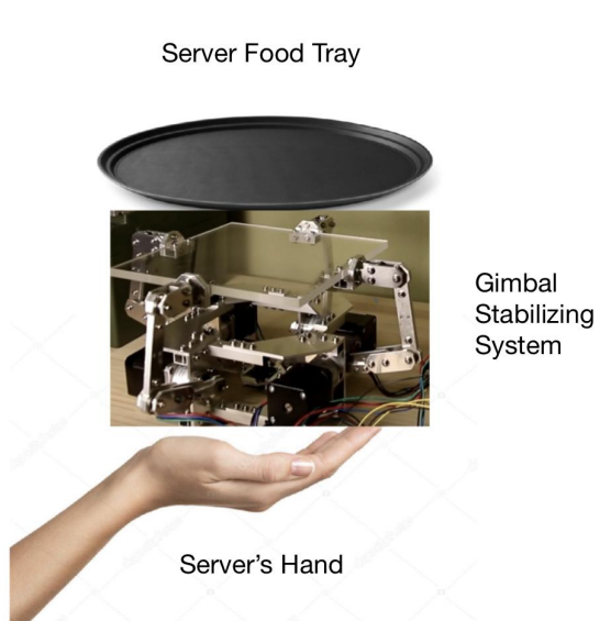
Initial Concept Design of Self-Balancing Food Tray
