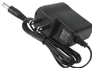
Figure 3: 5V Power Adapter
