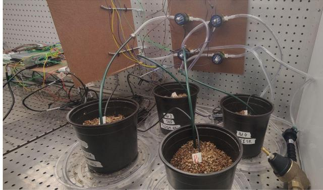
Figure 5: Irrigation system setup inside the growth chamber
