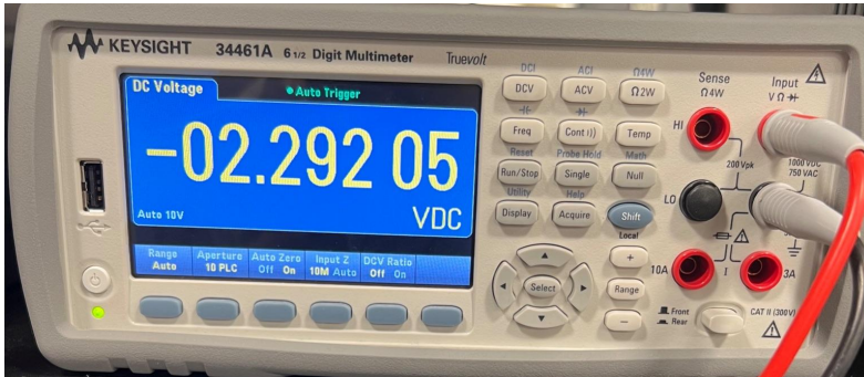
Voltage at Output of Vibration Motor GPIO pin
