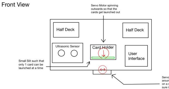
Servo Motor spinning around, but it's mounted on a steel base to make sure it's strong enough to rotate the whole device
