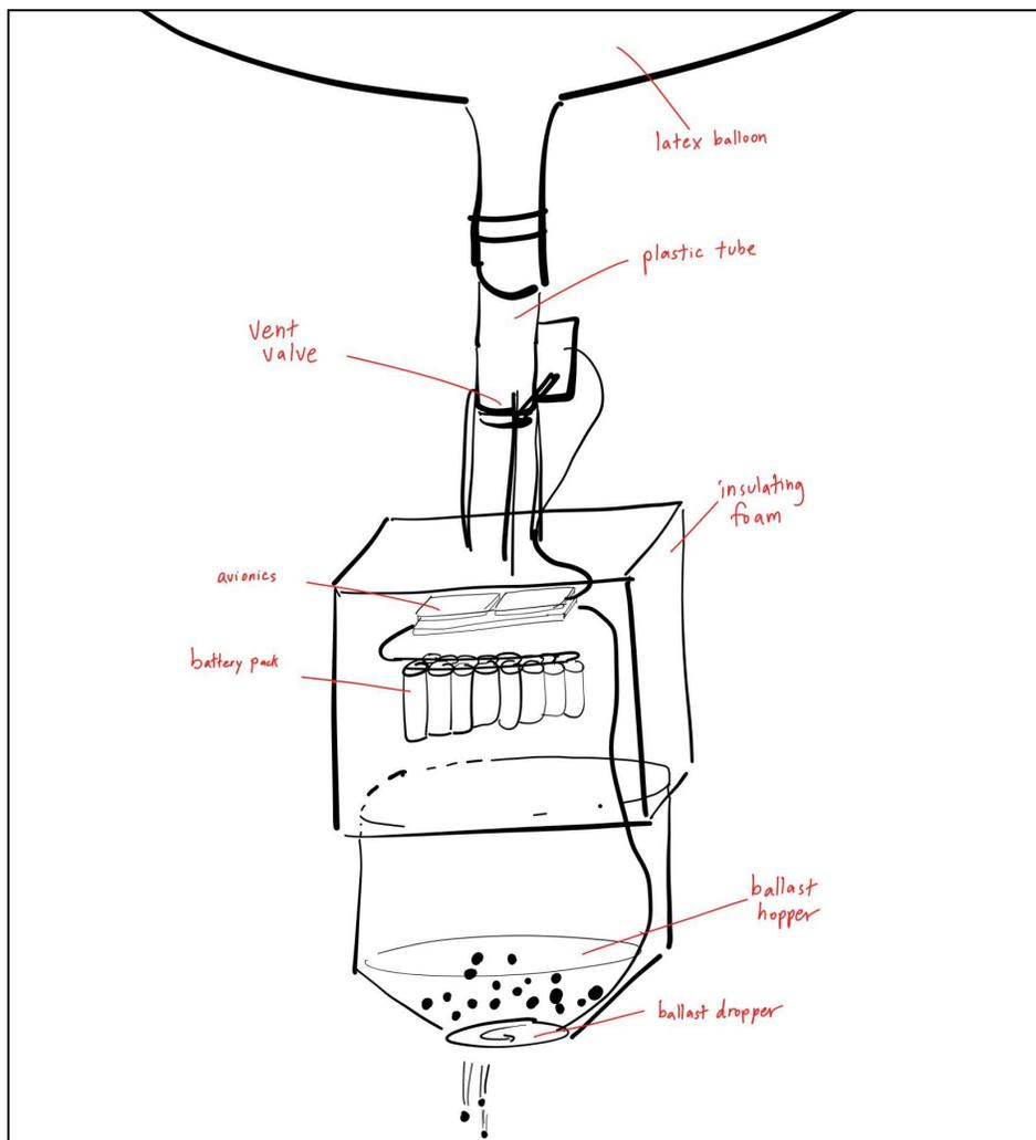
The entire system will be suspended from a plastic tube lashed to the opening of the latex weather balloon. The vent valve and its actuator is attached to the opening of the plastic tube. An insulating foam box is rigidly attached underneath the valve, where the avionics and battery pack is stored in a warmer environment. The avionics will consist of 3 boards: the main board that
