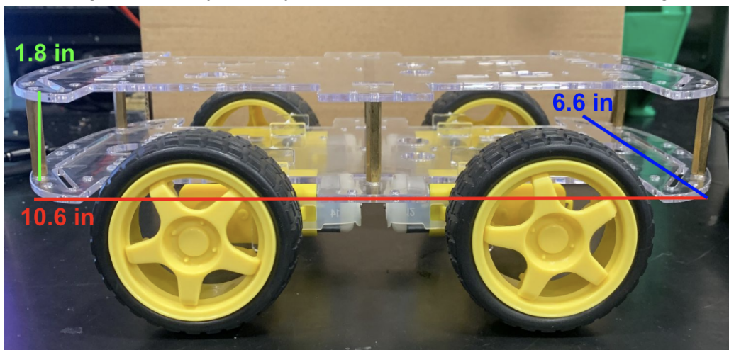
Figure 3: Physical dimensions of car chassis
