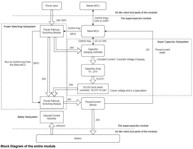
Legend: Thick arrows: Power Thin arrows: Data Rounded Rectangles: Off-the-shelf products Angled Rectangles: Customized circuits
