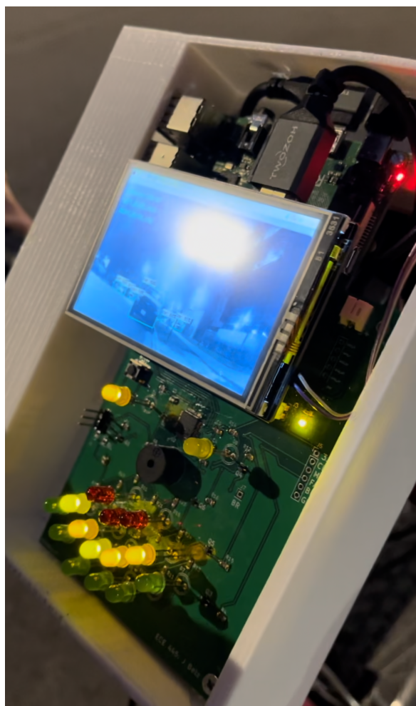
Figure 16: Night Condition Object Detection Verification
