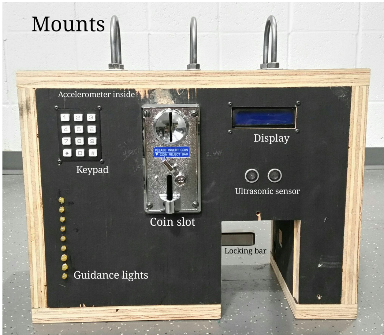
Figure 1: Photograph of the appliance, with interface elements labeled.
