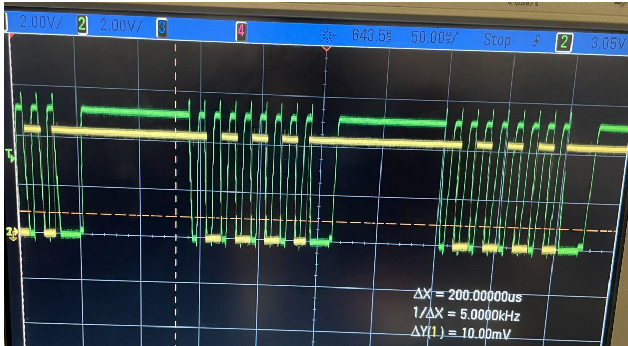
Figure 10: Response signal (yellow) on top of clock signal(green)
