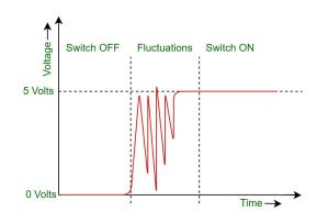
LED display and the circuit to act unusual for the first few seconds of turning on (Contributor, T. T.). Adding a debouncer should help "debounce" the signal so it does not turn on until it actually hits 5 volts. This way the signal is not interfered with and properly turns on when the user prompts it to.
