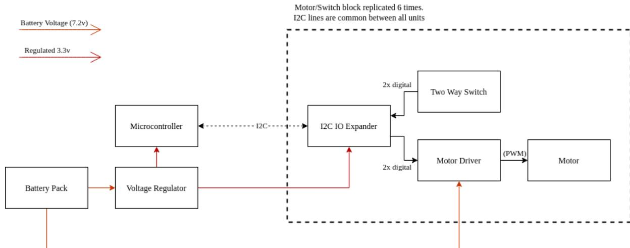
Figure 2: Block Diagram of Project Systems
