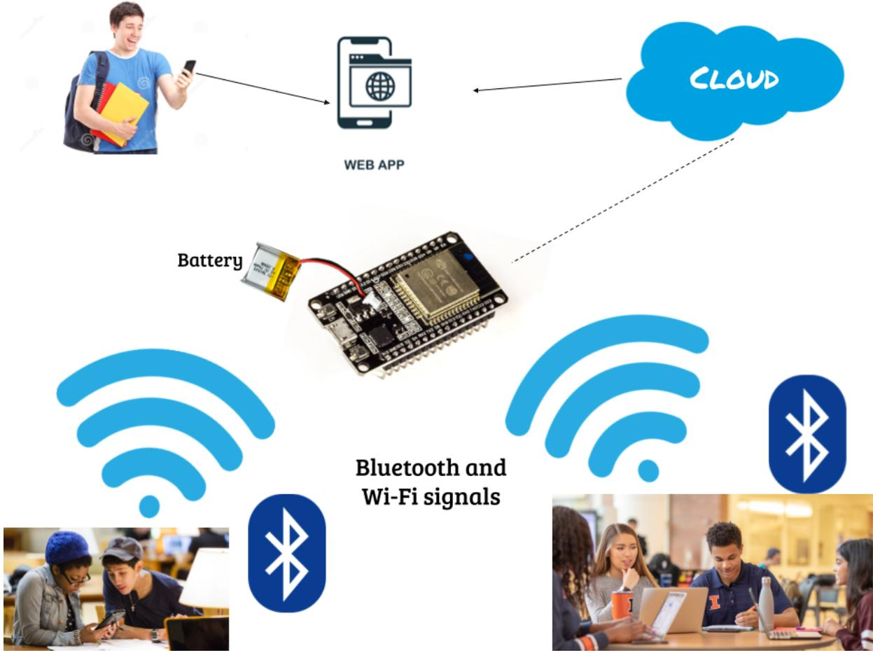
Figure 1: Interactions between nodes, student devices, and web application
