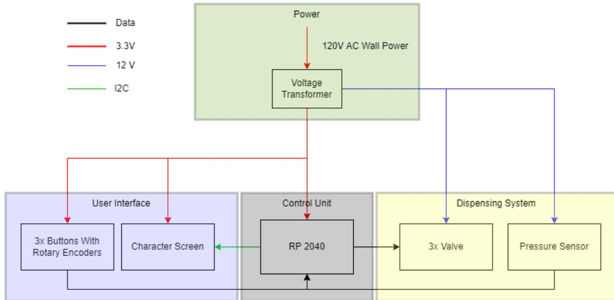
Figure 2: Block Diagram of Dispensing Machine
