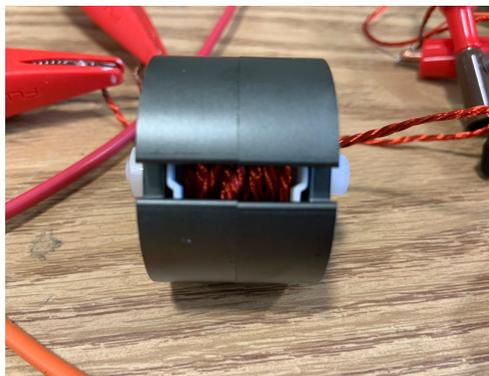
Figure 11 : Physical Construction of the Transformer
