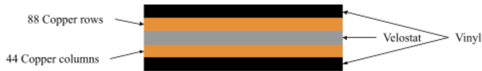
Figure 2: Side view of the layers of the pressure mat (not to scale)
