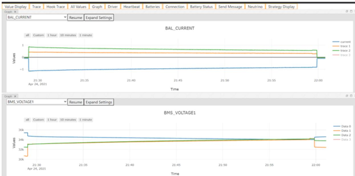
Figure 12: Telemetry capture of balancing currents and voltages during a 30 minute balancing test
