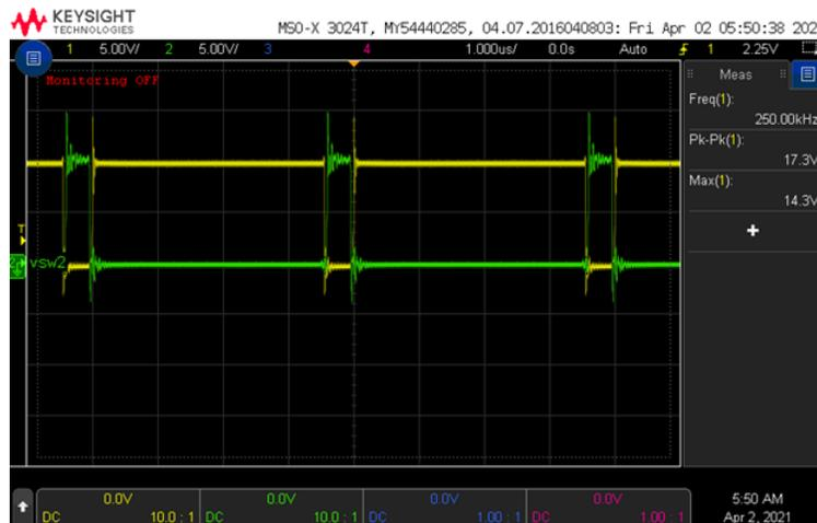
Figure 9: Oscilloscope capture of gate drive outputs
