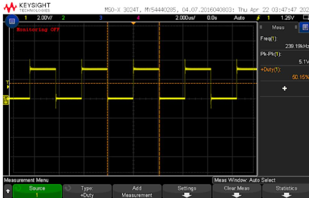
Figure 7: Oscilloscope capture of PWM output
