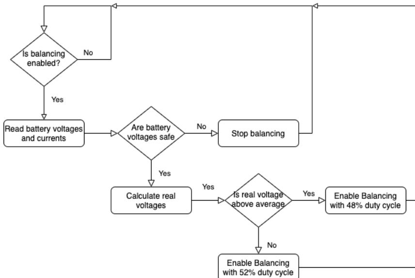
Figure 5: Balancing control algorithm
