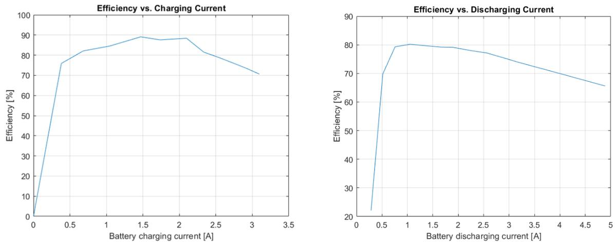
Figure 10: Efficiency characterization for flyback converter
