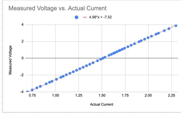
Figure 8: Linear regression of measured voltage versus actual current of current sense circuit for module 1
