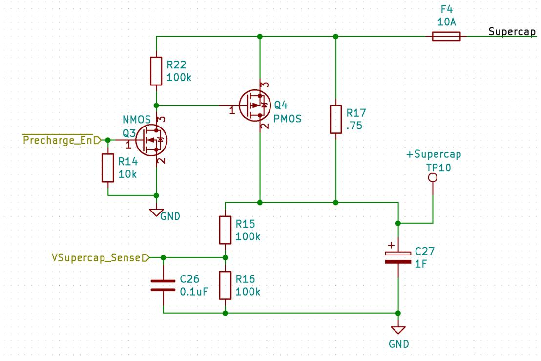
Figure 20: Schematic of precharge, supercapacitor, and voltage sense circuit
