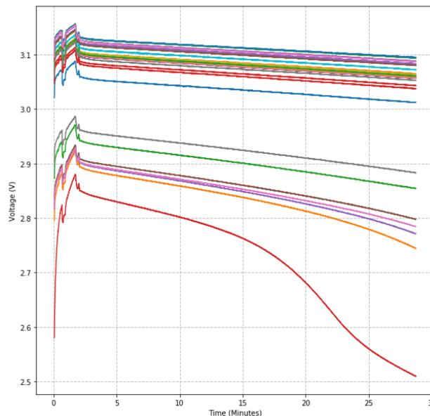
Figure 1: Module voltages during the last 30 minutes of the race. Each color represents a different battery module.
