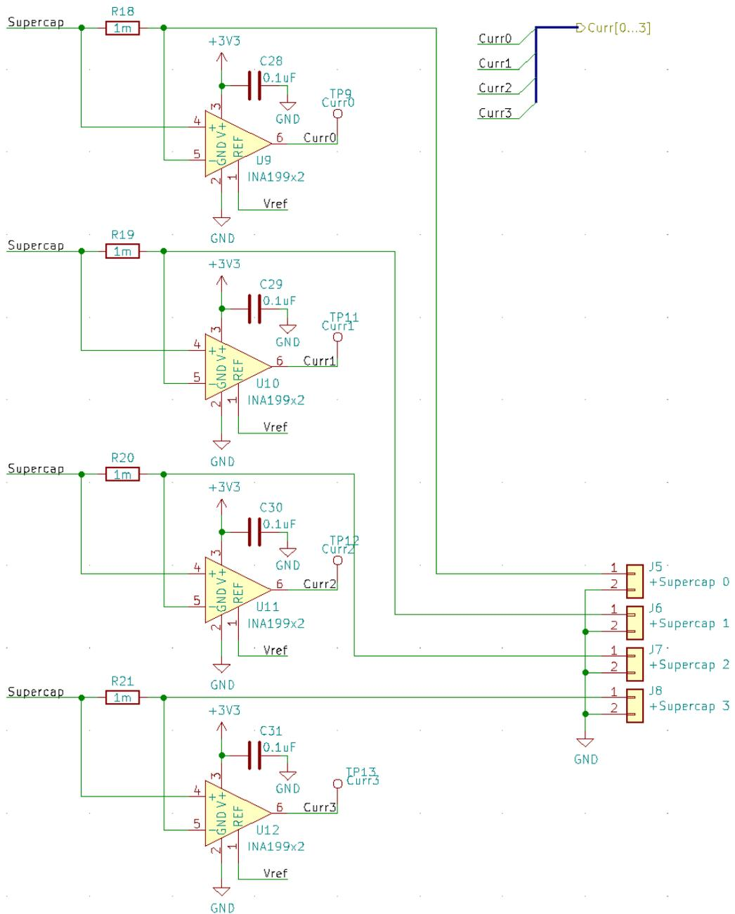
Figure 15: Schematic of current sense circuit
