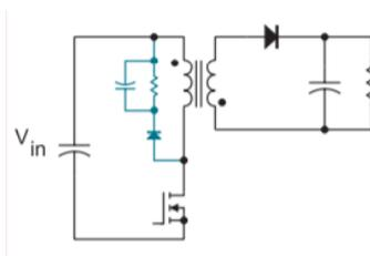
Figure 6: Schematic for an RCD snubber on a flyback converter
