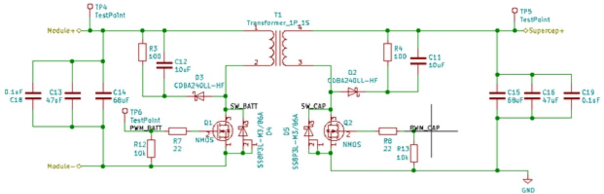
Figure 17: Full schematic of flyback converter
