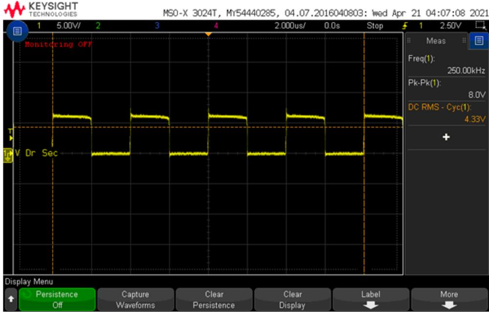
Figure 11: Oscilloscope capture of secondary drain voltage for 3.5 to 3.5 V conversion at 1.5 A load
