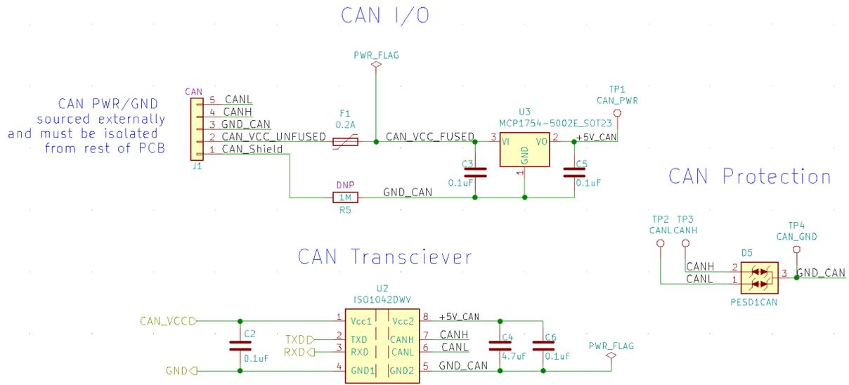
Figure 16: Schematic of CAN transceiver, input and output, and protection
