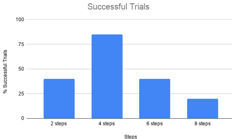
Figure 10: Chart of Successful Pill Dispensing by Motor Steps
