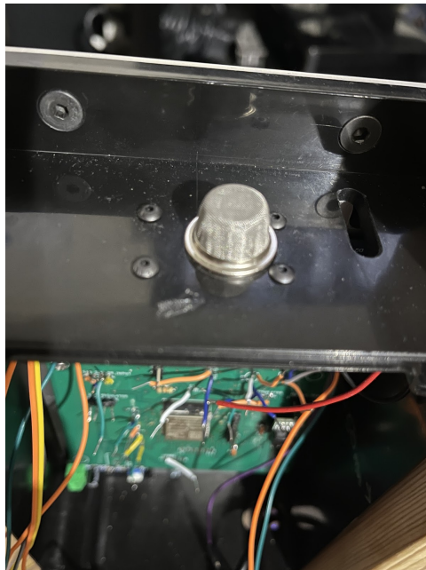
Figure 9: MQ2 Gas Sensor mounted above the black box.
