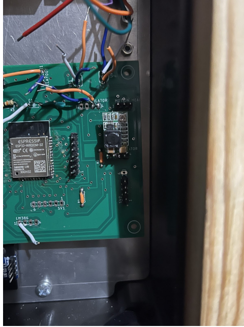
Figure 10: One of the voltage regulators on our PCB, used to distribute 12 Volts to the magnetic door lock.
