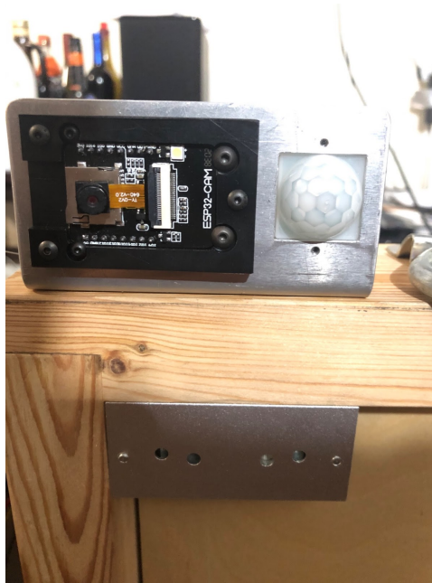
Figure 7: ESP32 Camera and Motion Sensor
