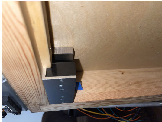
Figure 11: The magnetic door lock on the top of our door frame.
