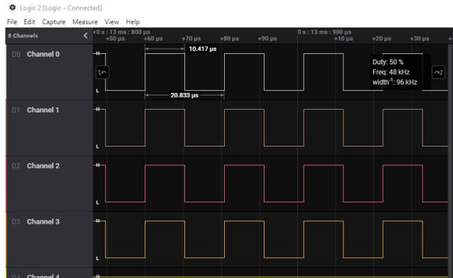
Figure 5: Logic analyzer trace showing four MEMS mics with synced clocks
