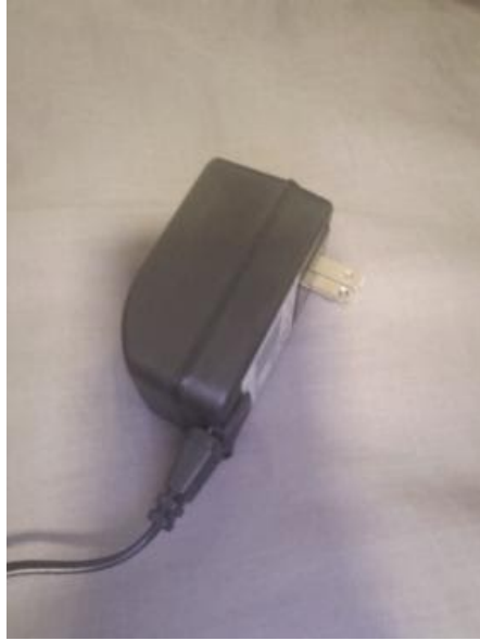
Figure 7: 120 VAC to 12 VDC Power Converter used in project
