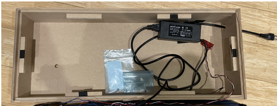
Fig. 3. Physical Appearance of Inside of Scoreboard
