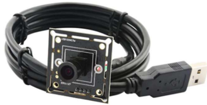
Figure 3 The ELP megapixel Super Mini 720p USB Camera web camera used in our design.
