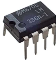
Figure 10 The LM-386N op-amp used in our design, which performs 20 times amplification by default.
