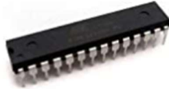
Figure 7 ATmega328p-pu microcontroller used in our design, which is the standard chip used in Arduino Uno.
