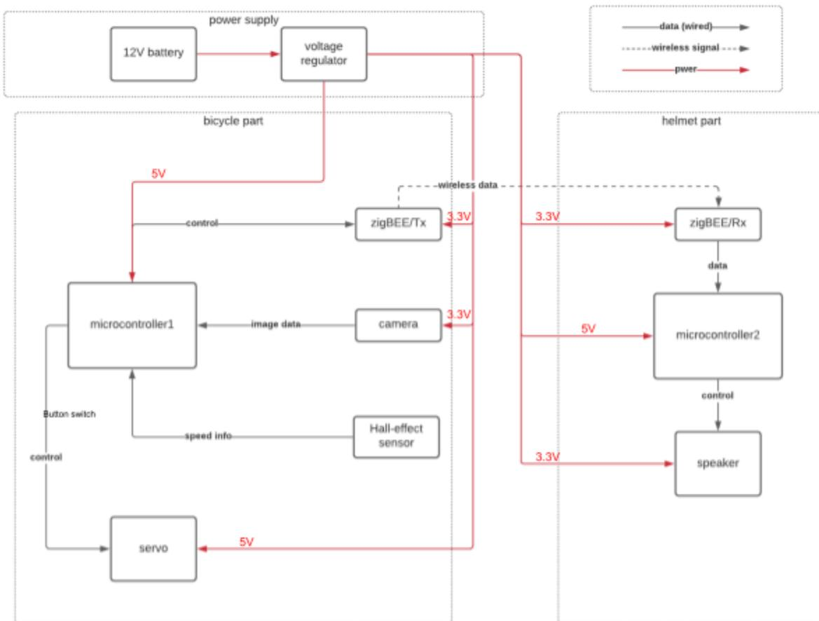
Fig.2 Block Diagram
