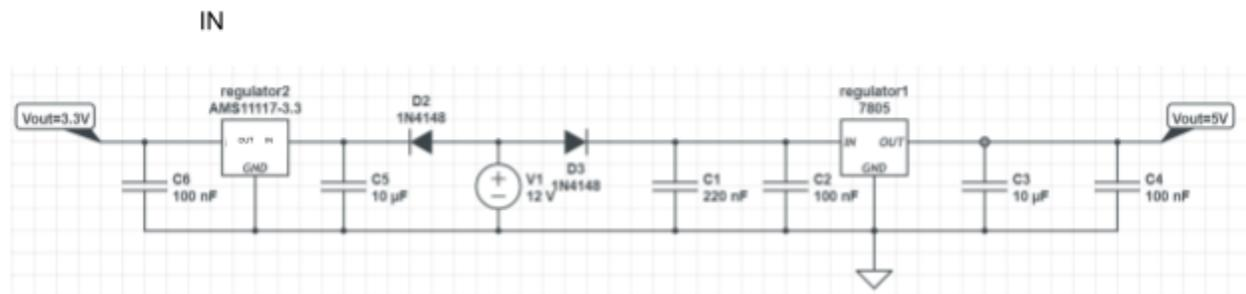
Fig.3 power supply circuit
