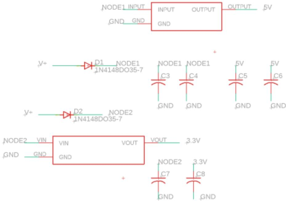
Fig.6 5V/3V power supply
