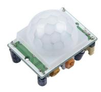
Above: Example of a passive infrared sensor
