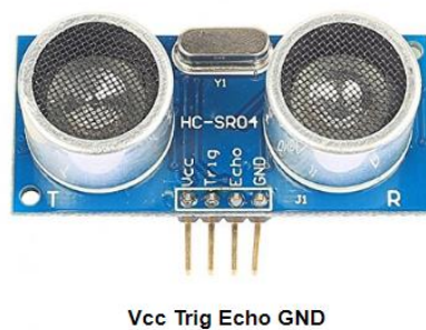
Figure 2.5 Ultrasonic Sensor and its pin out
