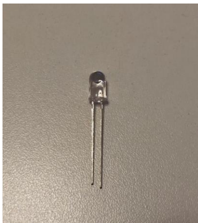
Figure 2.8 970 nm IR transmitter
