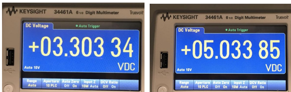
Figure 14. Output voltage of the 3.3V and 5V voltage regulator
