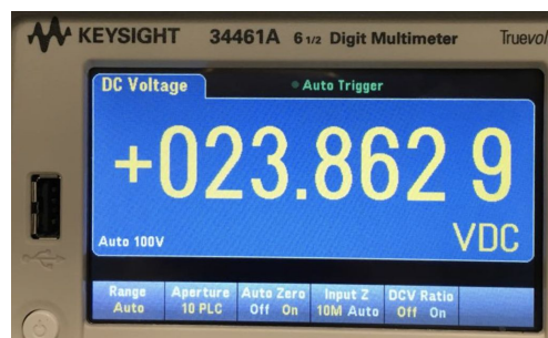
Figure 15. Output voltage of the 24V voltage regulator
