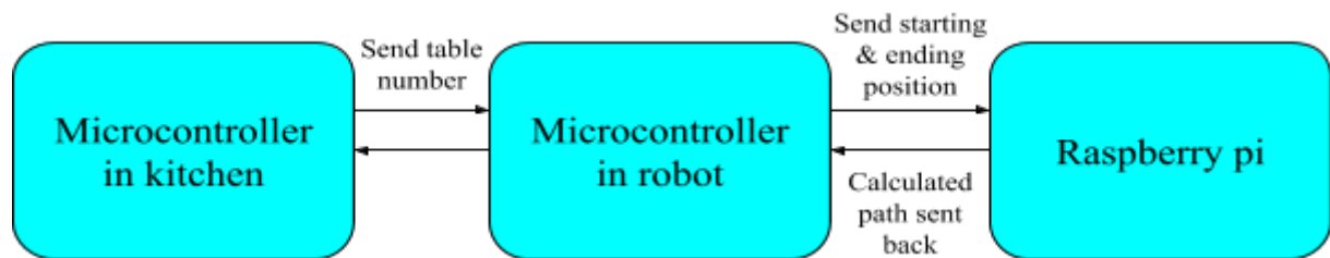
Figure 8. Overview of information relay in entire robotic waiter system
