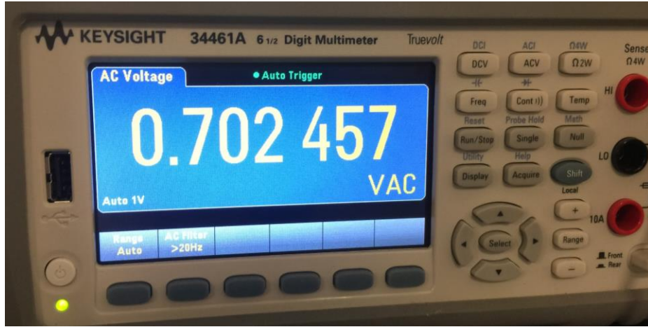
Figure 10: RMS Voltage across the Volume Control Knob
