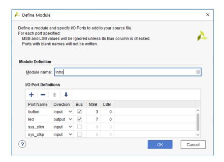
In this example, *button* is a 4-bit input signal; *led* is an 8-bit output signal; *sys\_clkn* and *sys\_clkp* are single bit input signals. These four signals are the input and output signals from the module that we will create shortly. They are also input/output signals from the FPGA to the outside world in this example. You will shorty create a constrains file which will define how these signals are mapped to physical pins on the FPGA.
