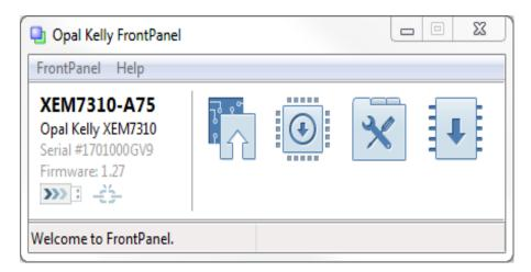
Click the middle-left button (IC with down arrow) and go to your corresponding project directory. Select the <FileName>.bit file, where <FileName> is your top-level filename. The FPGA should automatically flash and start running your program. Test it out by pressing button[0] on the board and see how the counter increments or decrements.
