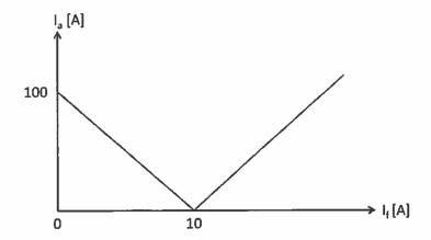
Find the equivalent circuit parameters (Kf and Xs)
