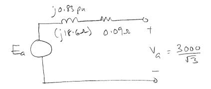
d) The motor is operated at rated voltage and current at unity power factor. Draw the phasor diagram for this case.
