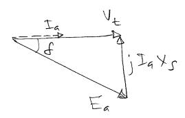
e) Re-draw the phasor diagram the leading power factor condition.
