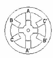
a) Plot the self inductance of phase 'A' as a function of rotor position, theta, starting in the position shown and rotated counter-clockwise. Superimpose with dashed lines and label the self inductance of phases 'B' and 'C'.
