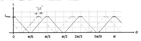
d. Plot the variation of torque versus rotor position,  $\theta$ , with constant current in Phase A. (Assume T<sub>max</sub> is known). Overlay in dashed lines, the variation of torque with constant current in Phase B.
