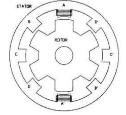
b. How fast would the rotor spin (in rpm) if excitation is applied at a frequency of one pulse per millisecond?
