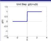
The derivative of the step function is the Dirac delta, which is not very useful in backprop.
