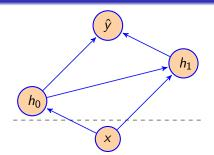
We often show the flow graph for the chain rule using bubbles and arrows, as shown above. You can imagine the chain rule as taking a summation along any cut through the flow graph—for example, the dashed line shown above. You take the total derivative from  $\hat{y}$  to the cut, and then the partial derivative from there back to x.
