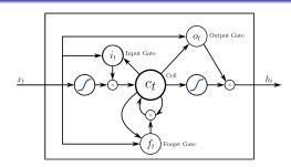
$$\begin{split} i[t] &= \text{input gate} = \sigma_g(w_i \times [t] + u_i h[t-1] + b_i) \\ o[t] &= \text{output gate} = \sigma_g(w_o \times [t] + u_o h[t-1] + b_o) \\ f[t] &= \text{forget gate} = \sigma_g(w_f \times [t] + u_f h[t-1] + b_f) \\ c[t] &= \text{memory cell} = f[t]c[t-1] + i[t]\sigma_h(w_c \times [t] + u_c h[t-1] + b_c) \\ h[t] &= \text{output} = o[t]c[t] \end{split}$$
