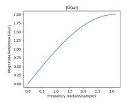
Frequency  $\omega = \pi$  means the input is  $(-1)^n$ :
