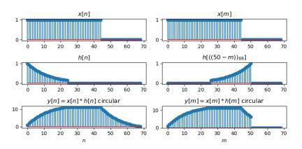
Case #2: n-m is negative, so it wraps around, but N is long enough so that the wrapped part of  $h\left[\left((n-m)\right)_N\right]$  doesn't overlap with x[m]
