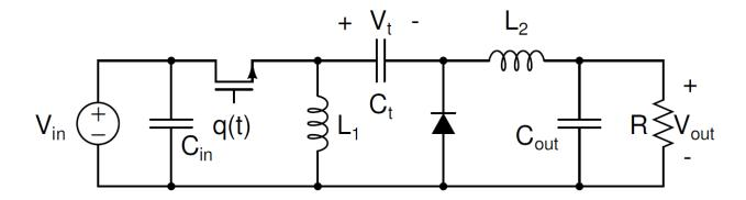
3. Consider an energy buffer for a 6-kW, level 2 onboard charger. The battery has a 400-V nominal voltage. The distribution grid operates at a frequency of 60 Hz and a peak voltage ripple of 8 V. **Determine** how large of a capacitor is needed to buffer the twice line-frequency power.
