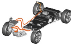
High Voltage Wiring
