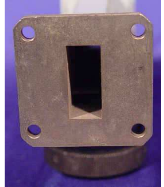
2.29 cm by 1.012 cm Standard X-band (8.2-12.4 GHz) waveguide in which only TE 10 mode is non-evanescent within X-band.
