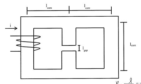
Draw the equivalent magnetic circuit.
