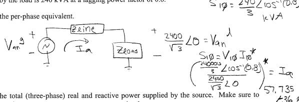
(b). Find the total (three-phase) real and reactive power supplied by the source. Make sure to include units.
